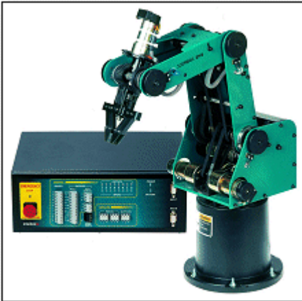
Robot arm capable of handshaking with mill
